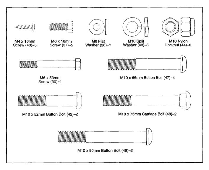
Identify the Front Stabilizer (2). While another person lifts the front of the Frame (1) slightly, attach the Front Stabilizer to the Frame with two M10 x 75mm Carriage Bolts (48) and two M10 Nylon Locknuts (44).
